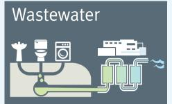
Wastewater, also known as sewage, is the used water that goes down sinks, washing machines, showers, baths and toilets. Most of it is water. The rest includes organic matter, such as human waste, food scraps, cooking fats, oil and grease, and debris, such as sand, grit and plastic.
